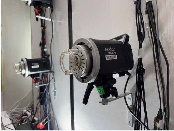
One of the 37 flashes behind the diffuser.
